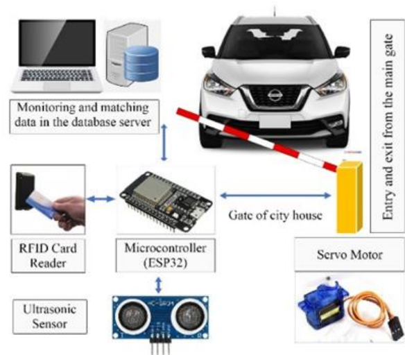
Figure 4 A general Working Diagram of Access Control System
